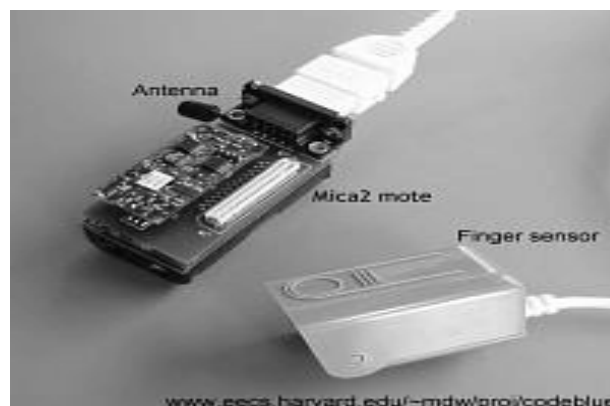
Fig. 2: A typical Mica2 mote used in CodeBlue[9]
